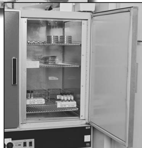
An incubator used to cultivate microorganisms
