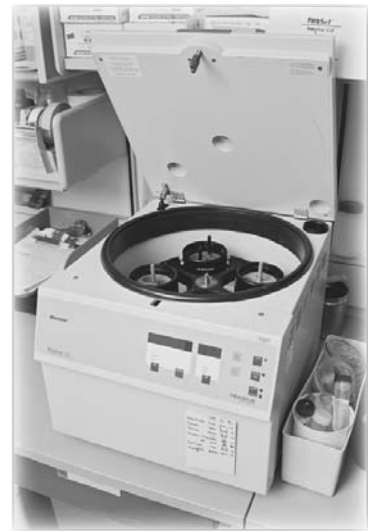
The centrifuge is used to prepare the sample.
