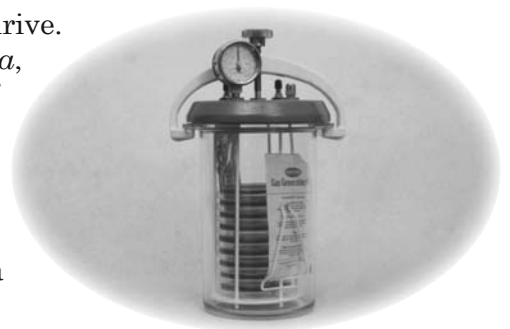
The gas pack anaerobic system
